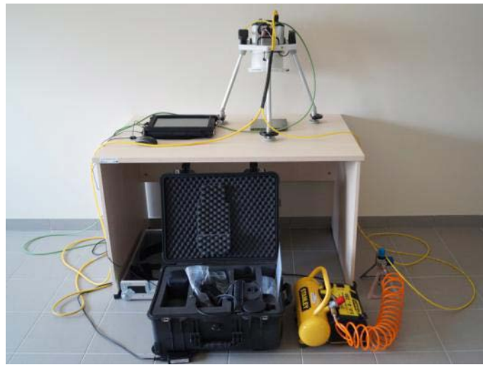
Figure 3: Mobile thermal imaging system for the inspection of composite structures
