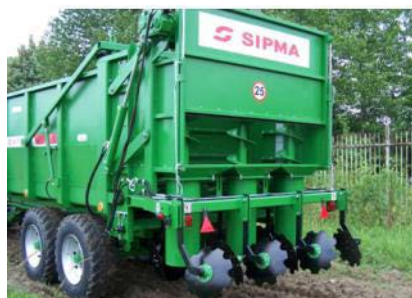
Figure 29: Functional model of a fertiliser dispenser for soil application of loose organic and mineral fertilisers (W.68444).
